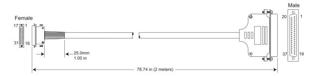
The TM-1400 camera uses the cable 30DG-02 from JAI PULNiX as a digital output cable. This cable has a 31-pin AirBorn connector on the camera end and a 37-pin D-sub male connector on the other end. Contact your JAI PULNiX representative regarding availability of interface cables for specific frame grabber models. Pinout configuration for the digital cable is shown below.
